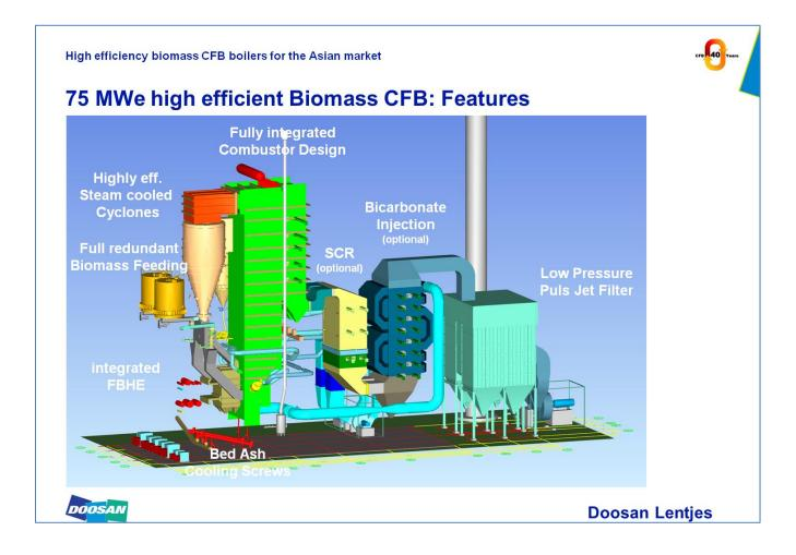
This CFB concept itself proved to sufficiently fulfil typical requirements on gaseous emissions without additional flue gas cleaning equipment (except bag house or ESP). Nevertheless, just in case due to specific local regulation very low emission limits are set up, the plant layout can be easily added by optional SNCR or SCR and lime or sodium bicarbonate powder injection to further reduce the low raw gas emissions of the biomass CFB combustion to figures of below 50
