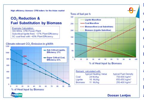
It is worse to note that cocombustion of about 20% of biomass in a 300 MWe CFB provides the same or even more CO<sub>2</sub> reduction single 60 MWe a as while biomass plant, combining the basic advantages of the utility size boiler e.g. utilizing high steam parameters and highly efficient steam
