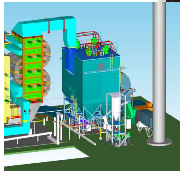
Biomass combustion, Sodegaura, Japan Electrical power: 1 x 75 MW Gas volume flow: 1 x 235,000 m 3 / h (STP, wet) FER-DI® flue gas cleaning
