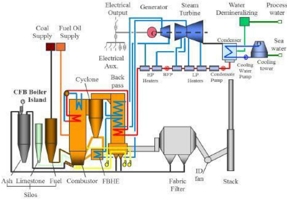
**Figure 1 – CFB Process Flow diagram (Sub-critical steam cycle)**
